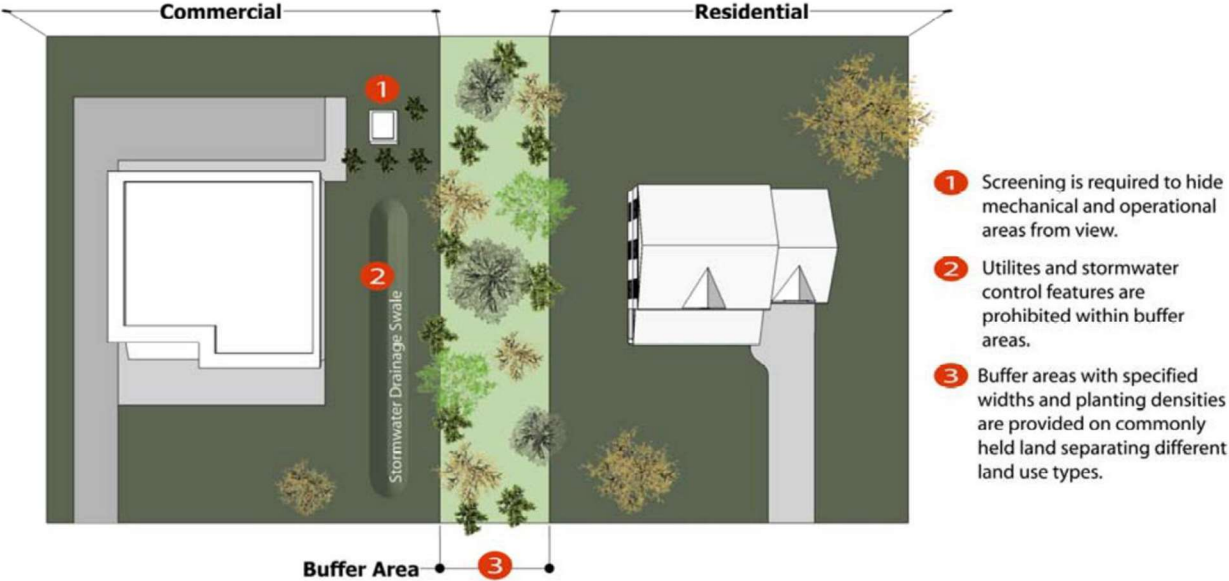
Figure 6-2: Required Buffer Placement
